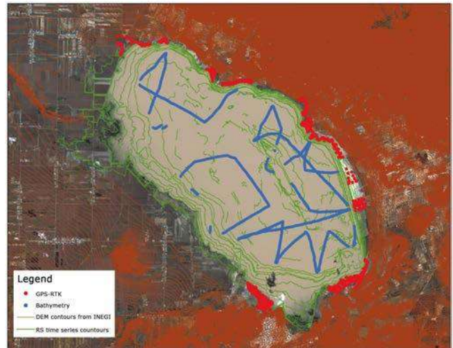
Figure 5. Map showing bathymetry, GPS points, derived curves from multispectral RS, and regional contours (INEGI).
